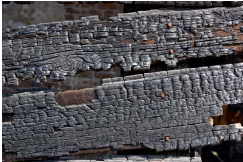
Fig. 13. Wood exposed to fire
