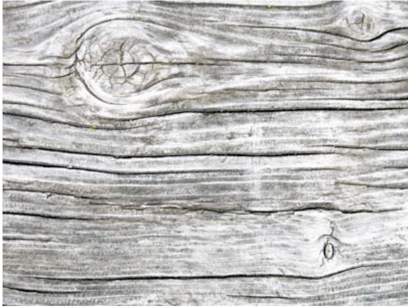
Fig. 12. Wood discoloured by the action of ultraviolet rays in sunlight.
